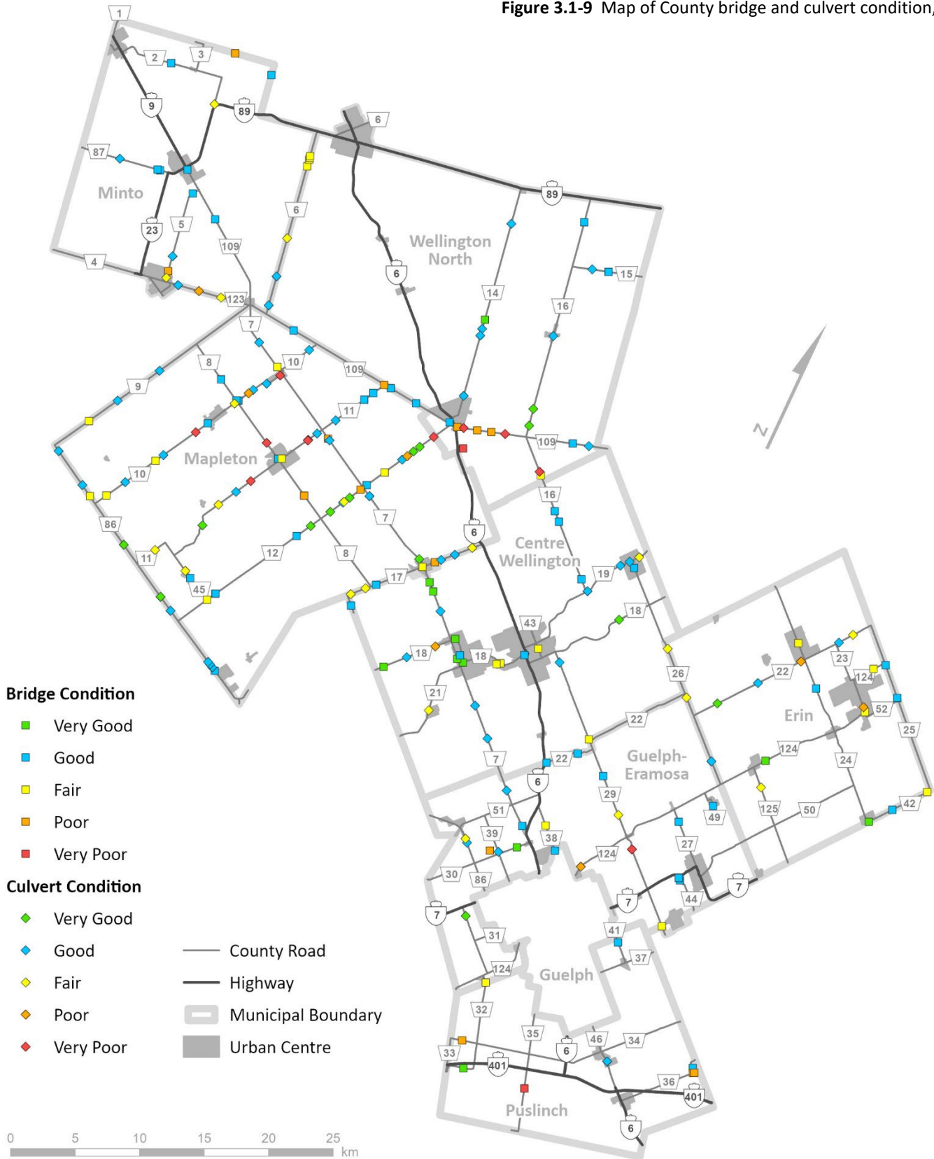
Figure 3.1-9 Map of County bridge and culvert condition, 2023.
