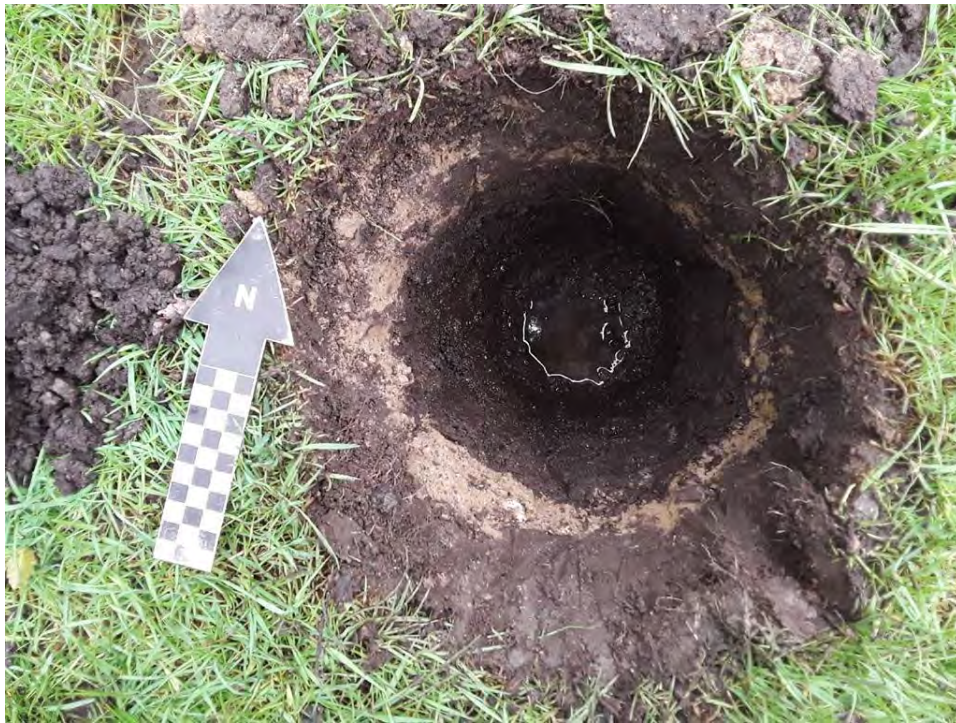
Image 27: A representative example of fill-capped wetland test pit stratigraphy in the central portion of the SE Site; facing north, May 19, 2022.
