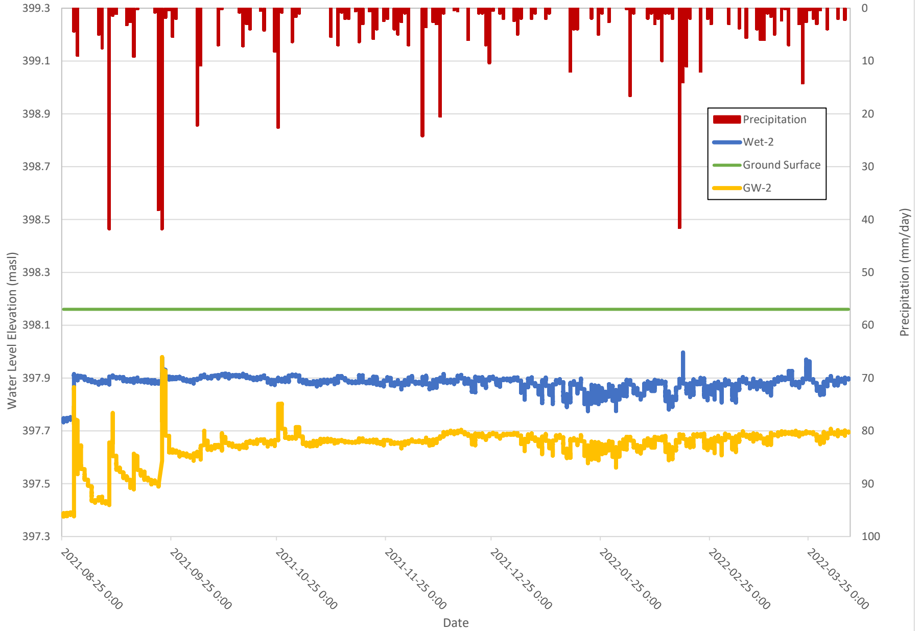
GW-2 and Wet-2 Water Level Elevation and Precipitation from August 25, 2021 April 5, 2022
