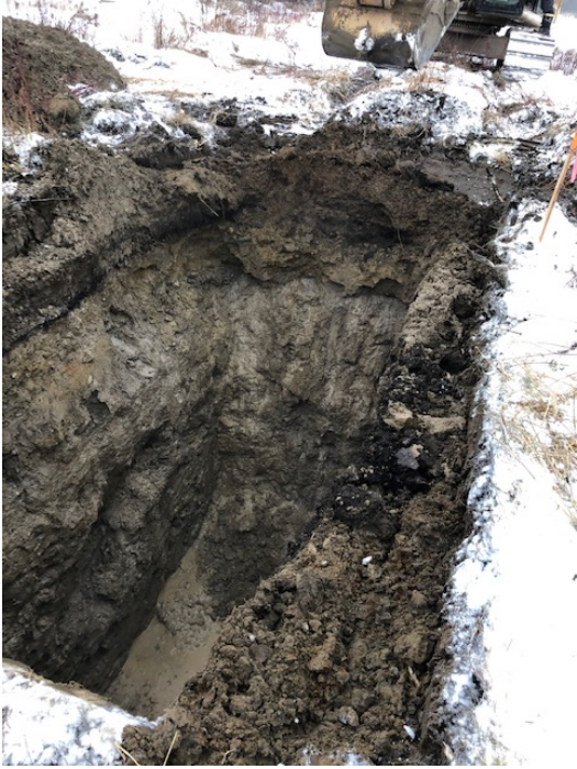
Photograph 11- View of excavation for TP 109. Water seepage was from sand and gravel seam at 2.0 to 2.5 m below existing grade.
