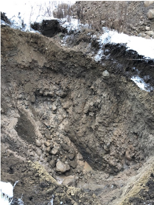
Photograph 6- View of excavation for TP 106. Note fast water seepage from sand and gravel seam at about 2.5 to 3.5 m below the existing grade.
