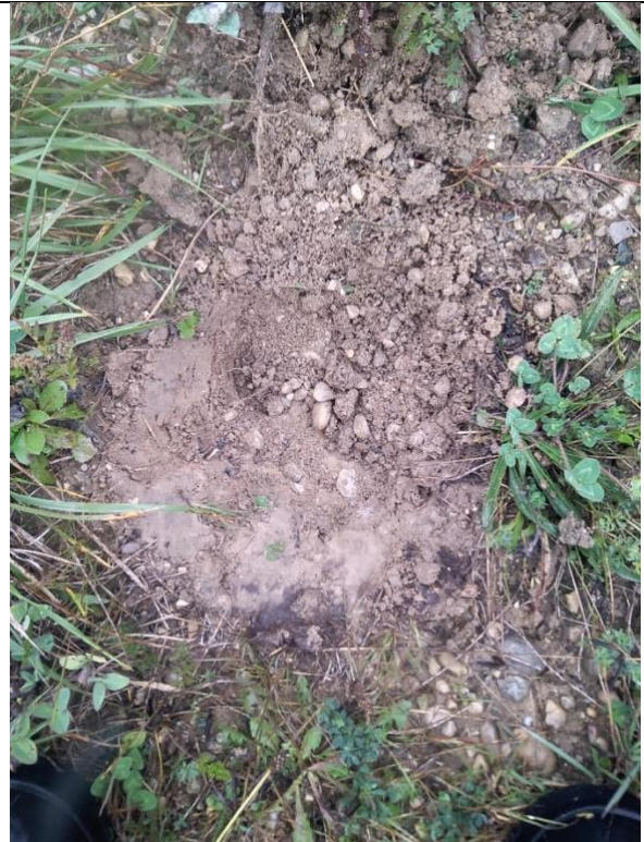
IMAGE 2 DISTURBED TP GRAVEL FILL
