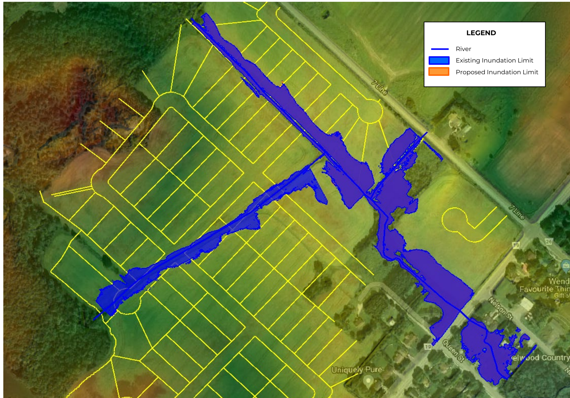
Figure 7.5: 12-hour Regional Storm Event Inundation Boundaries for Existing vs Proposed
