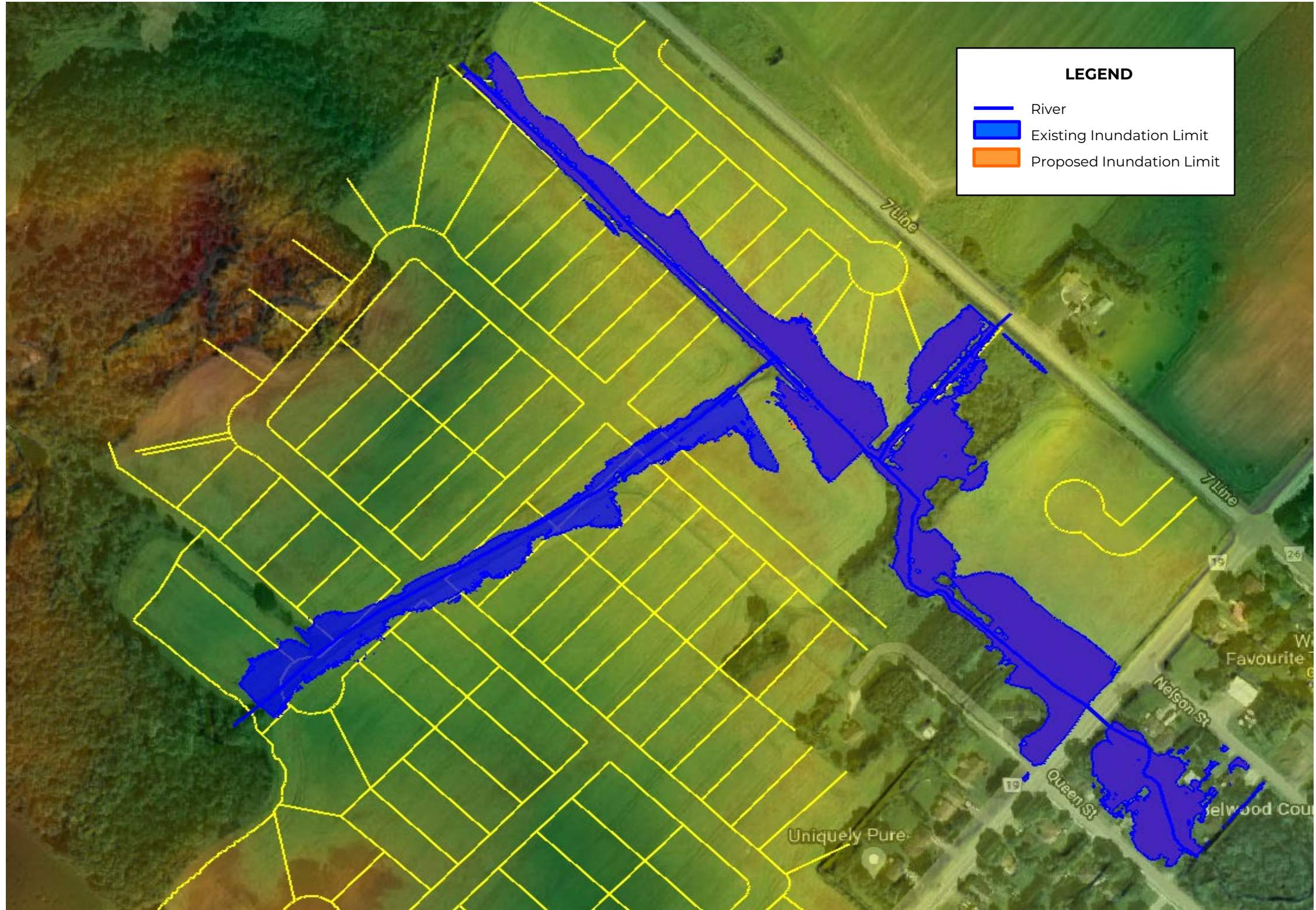
Figure 7.4: 100-year Storm Event Inundation Boundaries for Existing vs Proposed
