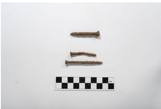
Plate 17: Metal Screw (T; Cat#187) and Wire Nails (B; Cat#186)
