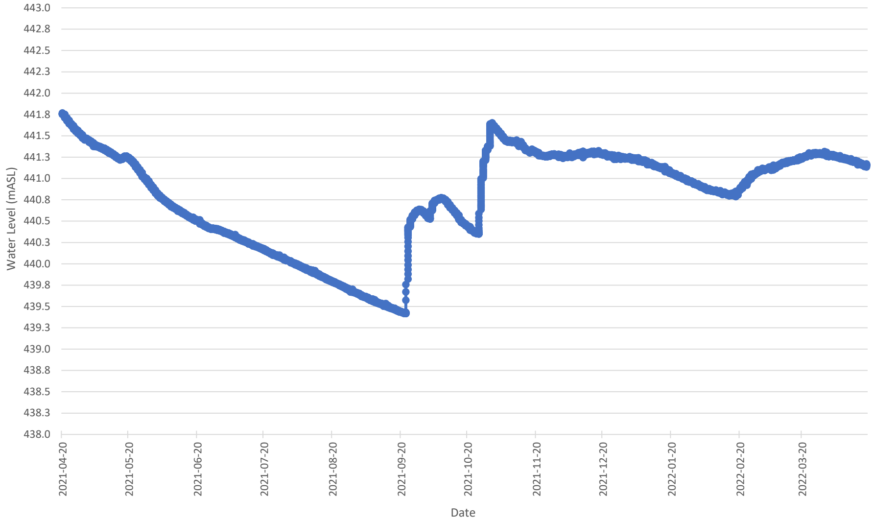
FIGURE 4 BH 01-20 - GROUNDWATER ELEVATIONS 31 Church Street, Alma, Ontario
