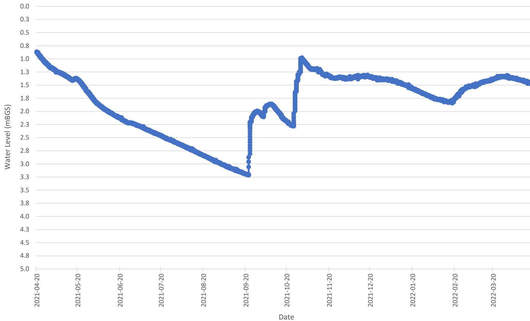
FIGURE 1 BH 01-20 - GROUNDWATER LEVEL MEASUREMENTS 31 Church Street, Alma, Ontario
