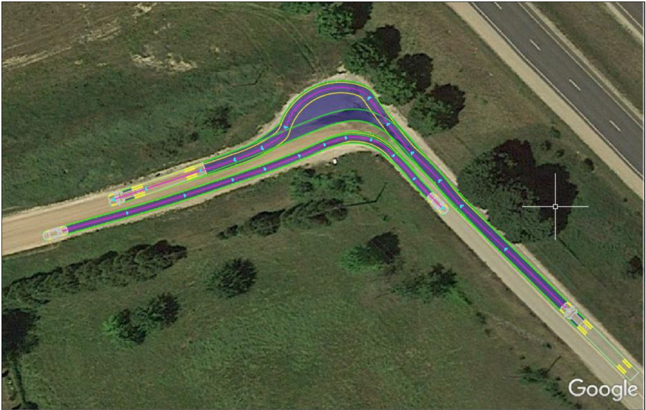
Figure 27 Westbound WB-20 Truck and Eastbound Passenger Car
