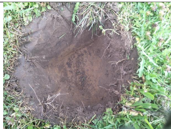
IMAGE 9 COMPLETED TEST PIT
