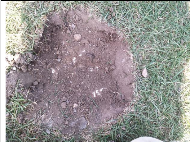
IMAGE 13 COMPACTED GRAVEL TEST PIT
