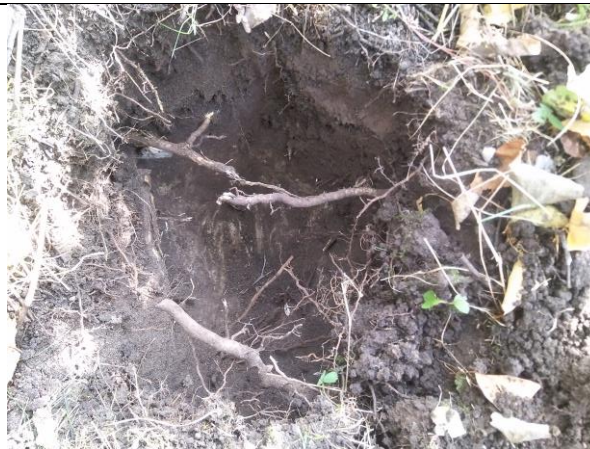
IMAGE 23 COMPLETED TEST PIT
