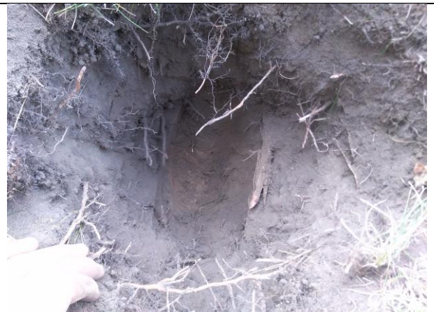
IMAGE 16 COMPLETED TEST PIT
